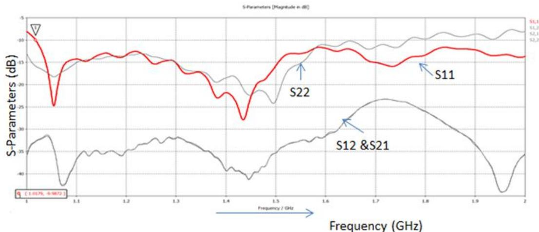
Figure 10. L-band antenna (Second model ports 1, 2)
