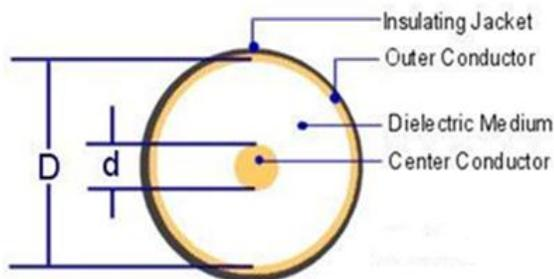
Figure 4. Cross section of coaxial line section
