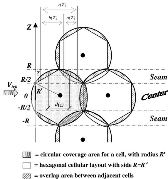
Figure 1. The shape of the cells and the distance crossed in the cell in the overlap area for a given height  $z$ .
