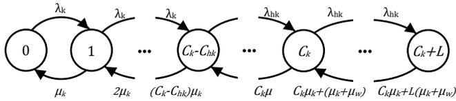
Figure 3. State Transition Diagram of CP Policy with Combination of Guard Channel and Handover Request Queuing Priority Scheme.
