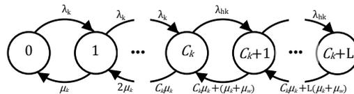
Figure 2. State Transition Diagram of CP Policy with Handover Queuing Priority Scheme.
