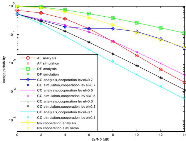
Figure 4. Outage probability for AF, DF and CC when shadowed Rician channel is in average shadowing.
