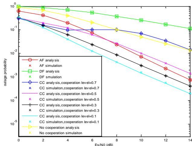
Figure 5. Outage probability for AF, DF and CC when shadowed Rician channel is in infrequent light shadowing.
