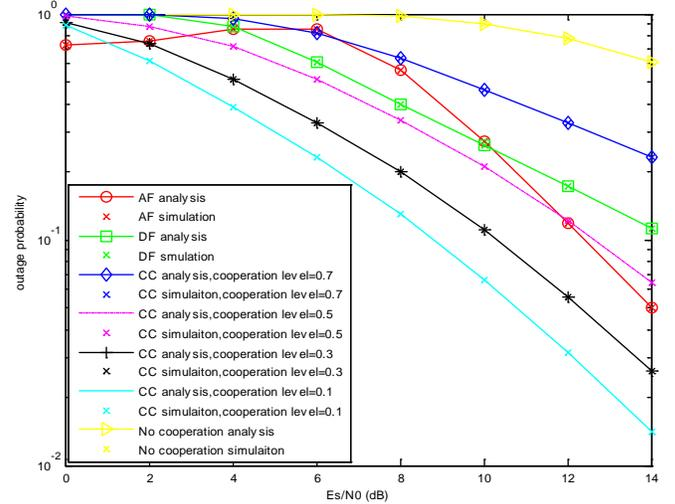
Figure 3. Outage probability for AF, DF and CC when shadowed Rician channel is in frequent heavy shadowing.
