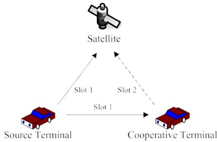
Figure 1. A three node LMS cooperative diversity system for AF and DF.
