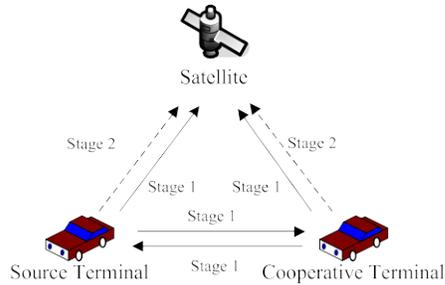
Figure 2. A three node LMS cooperative diversity system for CC.
