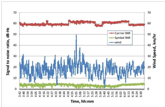
Figure 3. Signal SNR and wind speed measurements on DOY 241/2011 track with Kepler spacecraft at Ka-band.
