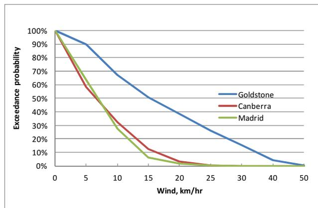
Figure 2. Exceedance probability distribution of wind speed at three tracking complexes.
