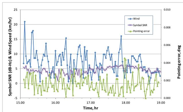
Figure 5. SNR, pointing error and wind speed on pass DOY 177/2011.
