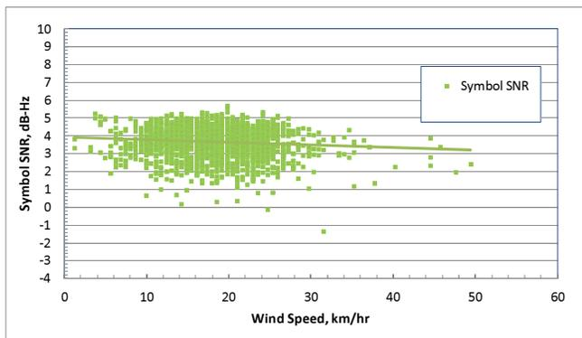
Figure 4. Correlation of symbol SNR against wind speed.
