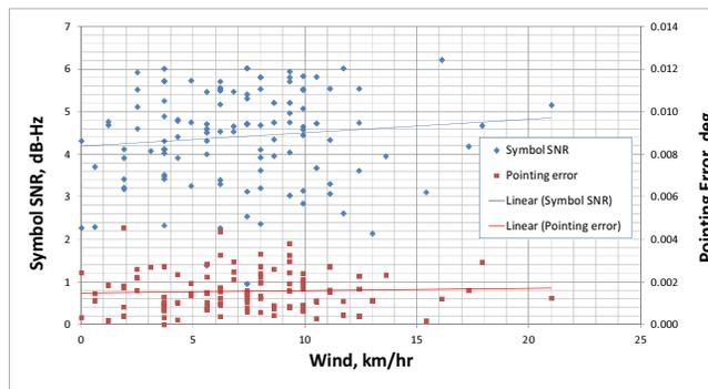
Figure 6. Correlation of received symbol signal to noise ratio and pointing error to wind speed.
