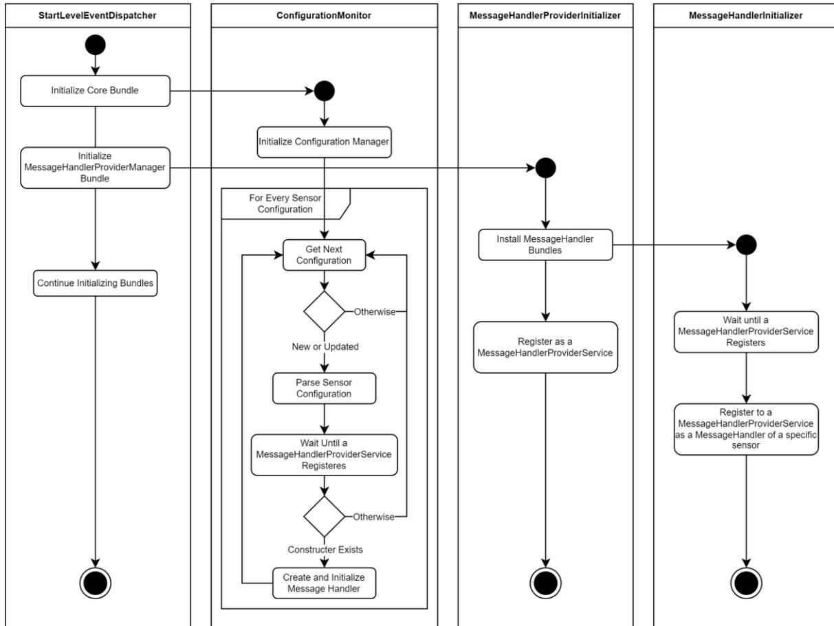
Figure 6. Message Handler initialization in the new architecture
