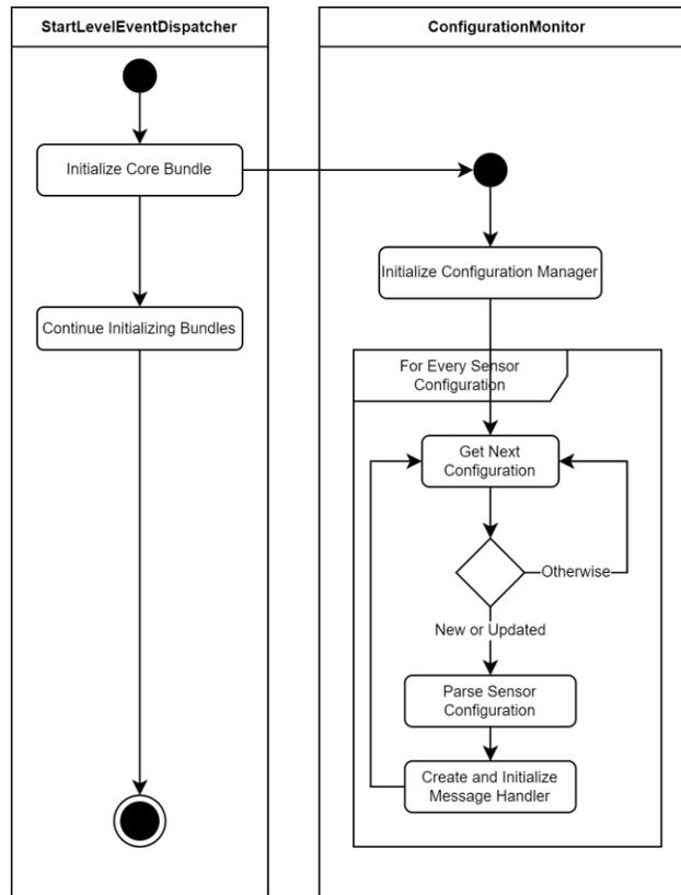
Figure 3. Message Handler initialization in the existing architecture
