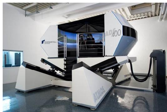
Figure 1. TRAFFIS-Full driving simulator operated by the University of Paderborn.
