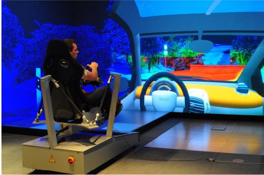
Figure 2. TRAFFIS-Portable driving simulator at the University of Paderborn.
