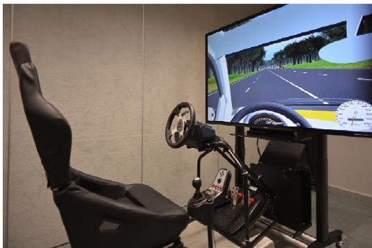
Figure 3. TRAFFIS-Light driving simulator at the University of Paderborn.
