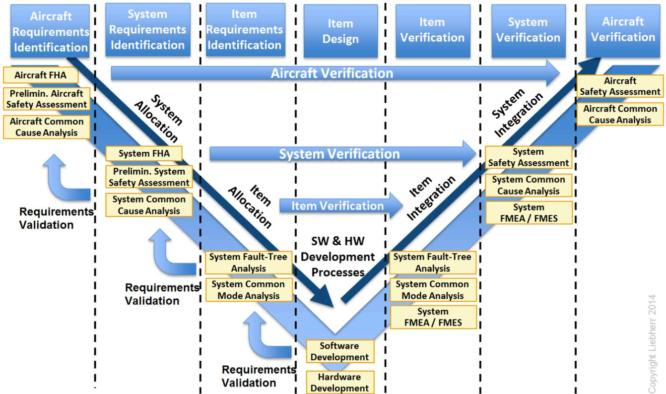
Figure 1: Avionics V-Model extract from the ARP4754A [12]
