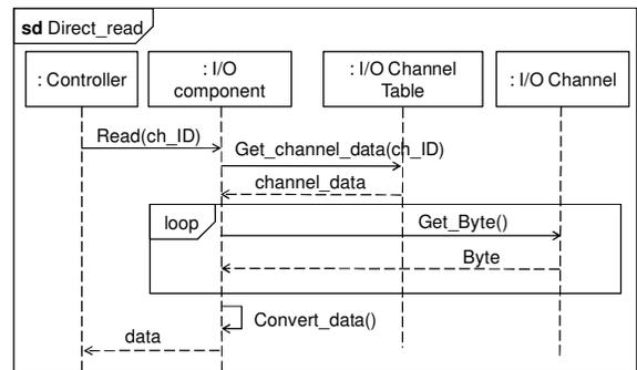
Figure 11. Process featuring direct access to I/O channels.
