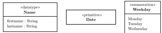
Fig. 7. Examples for datatypes in UML. Left: user-defined datatype with two components. Center: user-defined primitive datatype. Right: Enumeration with three allowed values.
