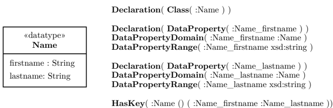
Fig. 11. Example for the transformation of a complex datatype.
