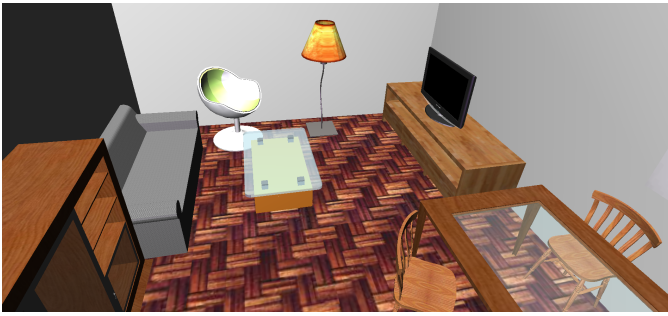
Fig. 9. Scene graphs allow the representation of hierarchical dependencies; As the TV is placed in dependence of the table, changing the table's position will also move the TV accordingly. Furthermore, scene graphs are memory efficient through instancing: the two chairs in this scene refer to the same geometry with different transformations.
