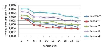
Figure 11. Energy consumption of single cluster head in reference to sender level
