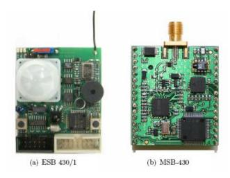
Figure 8. Sensor boards: ESB 430/1 and MSB-430
