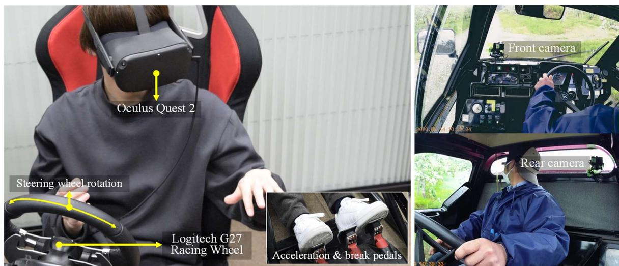
Figure 2. Sensors used in our VR simulator.
