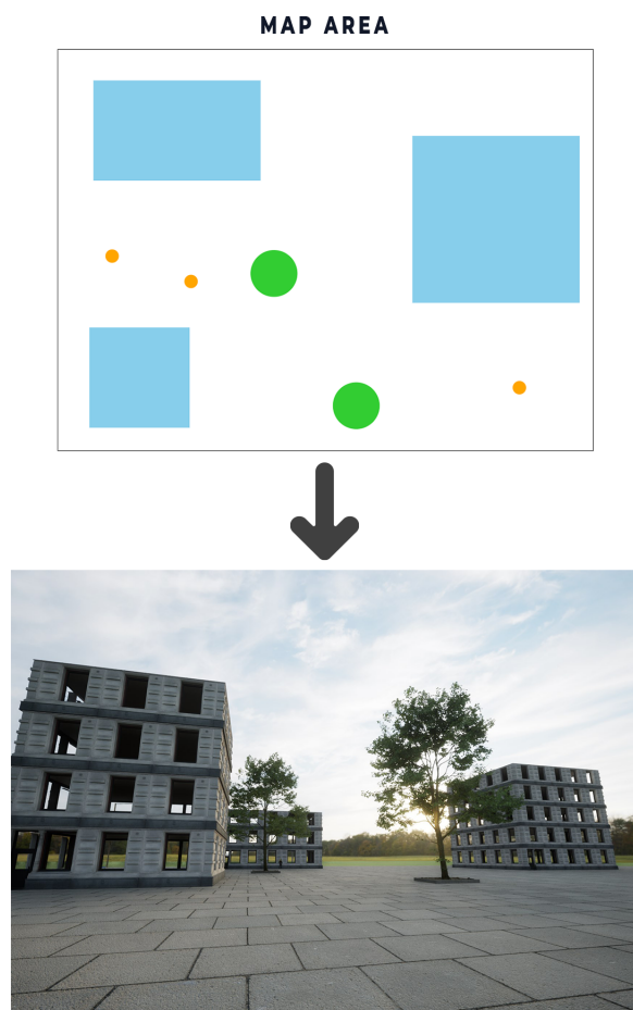
Figure 2. Top: Map created in browser-based authoring tool that exports Json. Bottom: Environment automatically recreated in Unreal Engine 5.1 after importing this Json file.
