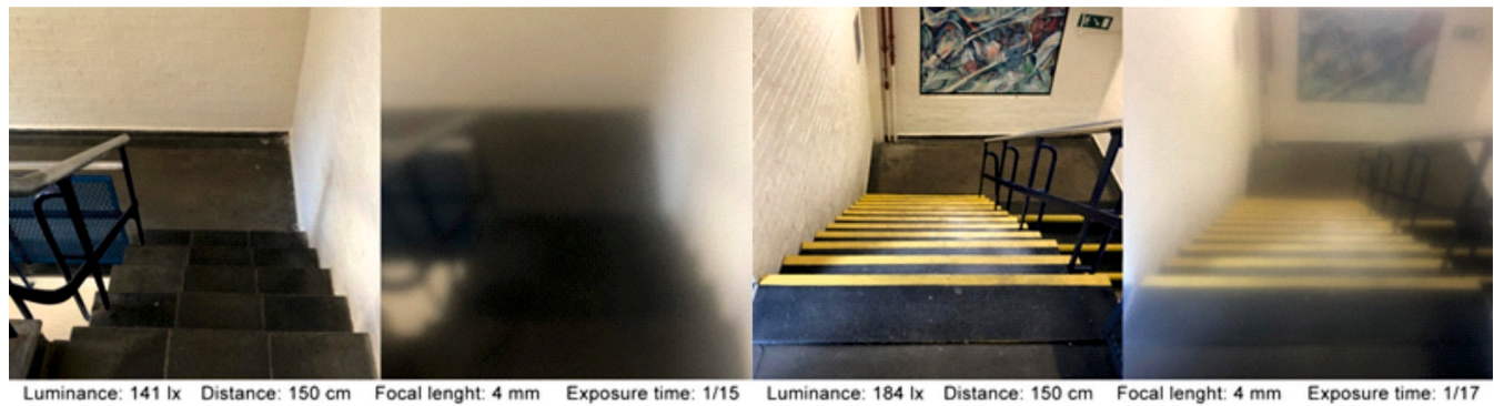
Figure 2. Staircase case study. From left: steps with no edging strip, without glasses (a) steps with no edging strip, with simulation glasses (b), steps with yellow edging strips, without glasses (c), steps with yellow edging strip, with simulation glasses (d).
