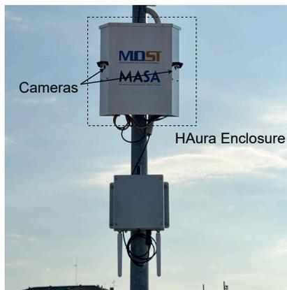
Figure 1. Haura hardware installed at the Modena Automotive Smart Area (MASA) [7]. Modena, Italy.
