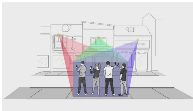
Figure 3. Combining transmitter swaths to achieve photonic cross-fire and a many-to-many network topology.
