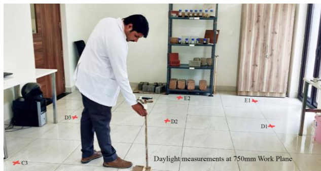
Figure 5. Measurements of illuminance levels using a Lux Meter at the MTCoE lab test bed
