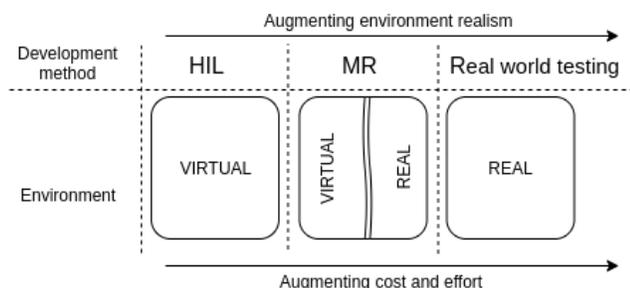
Figure 2. Environment in HIL architecture to MR [7].
