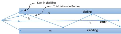
Figure. 1. Ray propagates when  $n_1 < n_2$  and  $angle > criticalangle$
