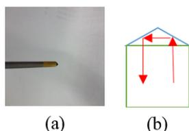
Figure 7. (a) The real fiber used to build the simulated diamond head (b) Ray reflected from the diamond head back to the fiber
