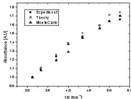
Figure 5. Average Relative Absorbance for Fiber with Narrowed Midsection [2]
