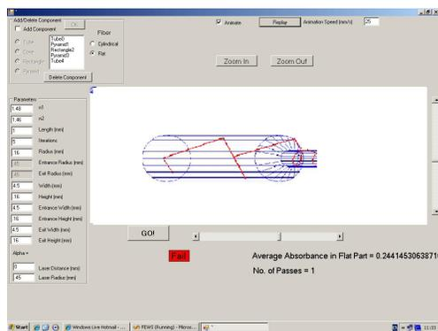
Figure 4. The first software simulation tool
