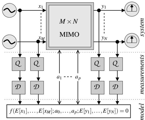
Figure 1. Modeling and measurements of a static ( $M \times N$ ) MIMO system.
