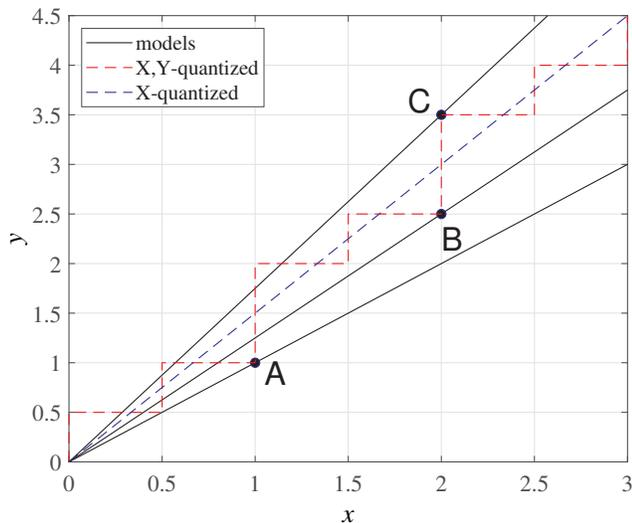
Figure 2. The consequences of the input-output uniform quantization on modeling linear SISO systems.
