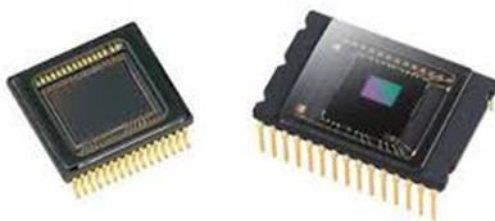
Figure 5. Example of CCD (left) and CMOS (right) sensor [20].
