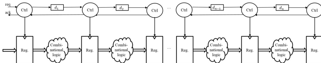
Figure 3. Architecture of an  $n$ -stage micropipeline
