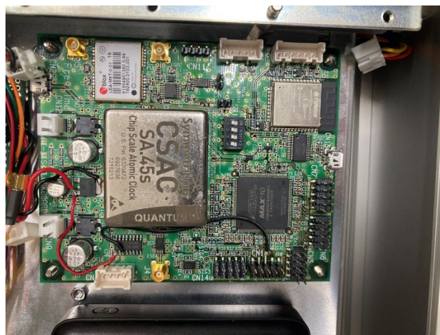
Figure 3. External appearance of oscillator and FPGA.
