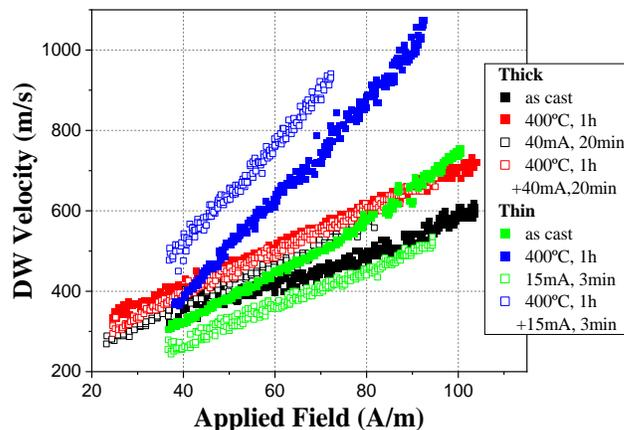
Figure 4. DW velocities of samples after annealing.
