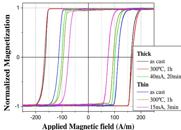
Figure 1. Hysteresis loops of samples before and after different treatments.
