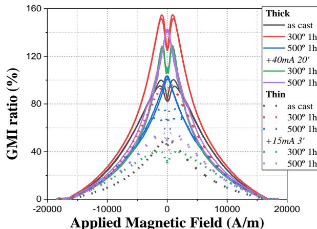
Figure 5. GMI ratios of microwire samples at 200 MHz.
