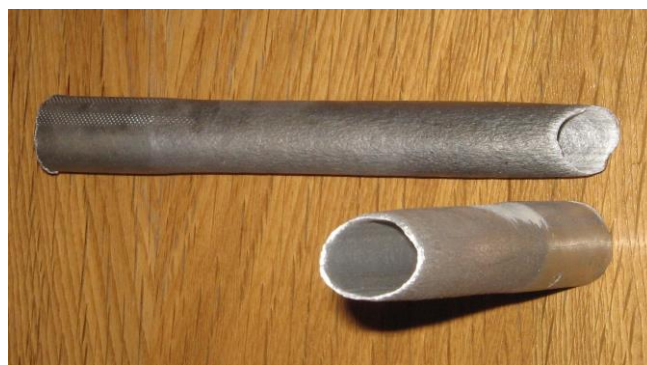
Figure 10. Broken aluminium pipe at maximum mechanical stretch.
