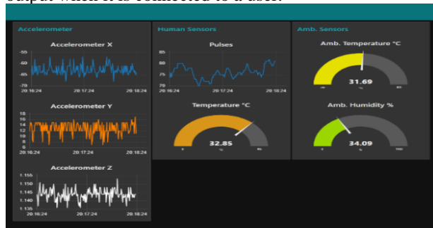
Figure 3. UI FRED, showing real time measurements of the fabricated Internet of Things wearable device.
