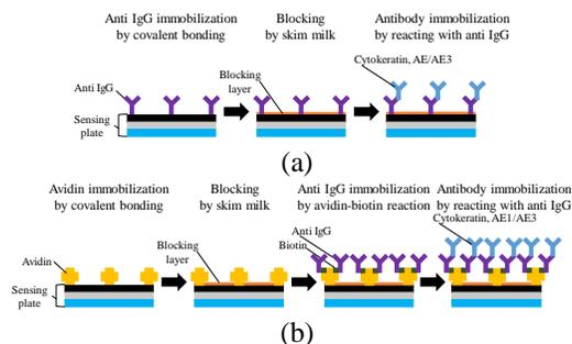
Figure 1. The processes of immobilizing antibodies on the SiO<sub>2</sub> film surface on the sensing plate: (a) Covalent bonding method (b) avidin-biotin reaction method
