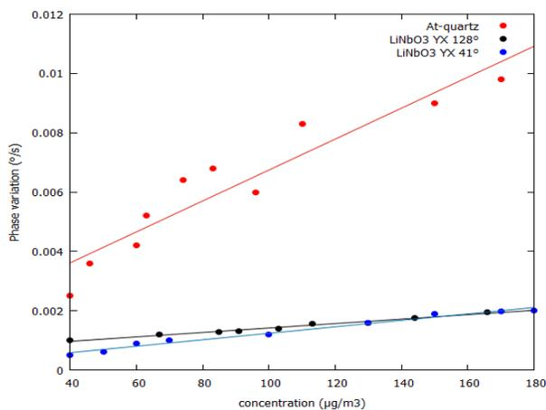
Figure 2. Phase derivative of SAW sensors based on AT-Quartz substrate (red)  $128^\circ$  YX  $\text{LiNbO}_3$  substrate (black) and  $41^\circ$  YX  $\text{LiNbO}_3$  substrate as a function of PM10 concentration.
