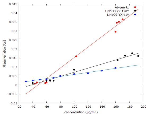
Figure 1. Phase derivative of SAW sensors based on AT-Quartz substrate (red)  $128^\circ$  YX  $\text{LiNbO}_3$  substrate (black) and  $41^\circ$  YX  $\text{LiNbO}_3$  substrate as a function of PM2.5 concentration.
