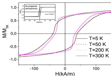
Figure 7. Hysteresis loops of annealed at 500 °C for 1 h  $Fe_{50}Pt_{40}Si_{10}$  microwires measured at different temperatures. Hysteresis loops of as-prepared are provided in the inset Adapted from Ref. [46].
