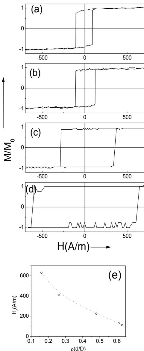
Figure 2. Hysteresis loops of  $Fe_{70}B_{15}Si_{10}C_5$  amorphous microwires with different metallic nucleus diameter  $d$  and total diameters  $D$ : with  $\rho = 0.63$ ;  $d = 15 \mu m$  (a);  $\rho = 0.48$ ;  $d = 10.8 \mu m$  (b);  $\rho = 0.26$ ;  $d = 6 \mu m$  (c);  $\rho = 0.16$ ;  $d = 3 \mu m$  (d) and  $H_c(\rho)$  dependence of the same microwires(e).
