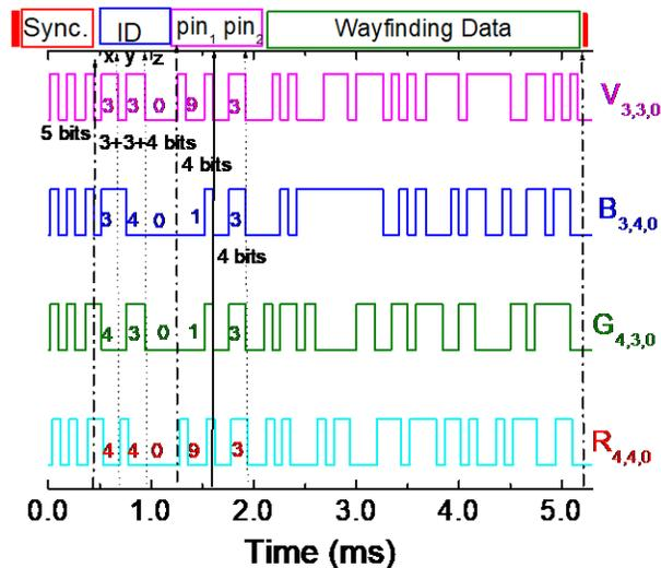
Figure 3 .Data frame structure. Representation of one original encoded message, in a time slot:  $R_{4,4,0}$ ;  $G_{4,3,0}$ ;  $B_{3,4,0}$  and  $V_{3,3,0}$  are the transmitted node packet from the unit cell  $C_{4,3,0}$  in the network.
