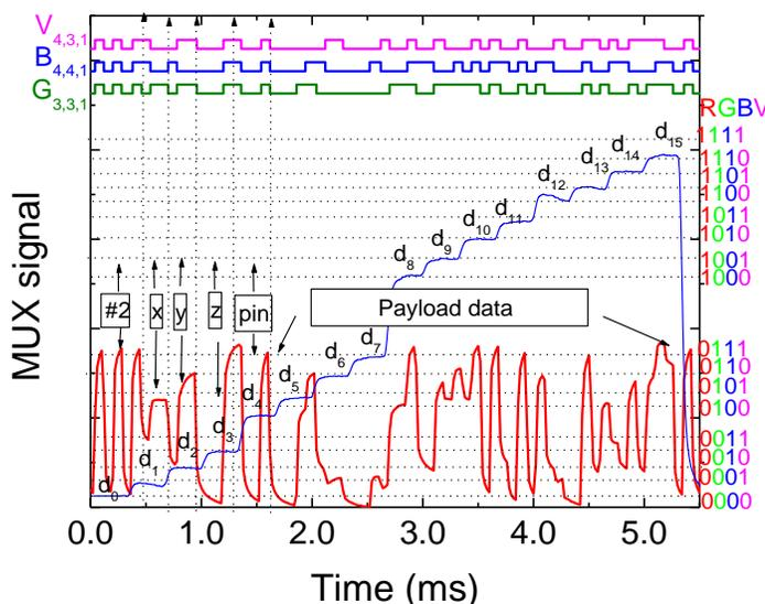
Figure 4 MUX/DEMUX signals received in the first floor in cell  $C_{4,3,1}$  footprint #6. On the top the received information is decoded. The MUX signal of the calibrated cell in the same frame of time is superimposed
