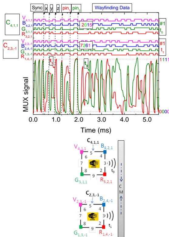
Figure 6 . MUX/DEMUX signals assigned to a “request”. MUX signal received by the CM receiver from two users (“2015” and “7261”) at different locations ( $C_{4,1,1}$ ; #1 and  $C_{2,3,-1}$ ; #1 ) in successive instants ( $t_0$  and  $t_1$ ). On the top the transmitted channels packets are decoded [Xi,j].
