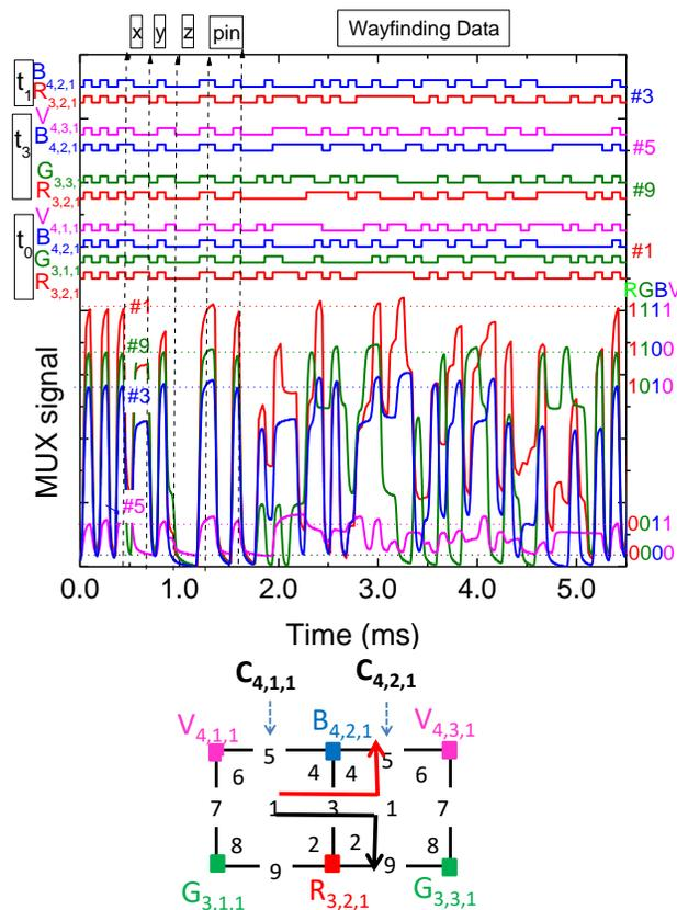
Figure 5 Fine-grained indoor localization and navigation in successive instants. On the top the transmitted channels packets are decoded [R, G, B, V] in the successive instants.
