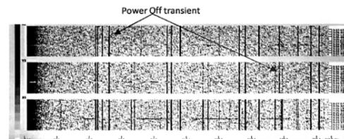
Figure 3. Waterfall display of frequency density.
