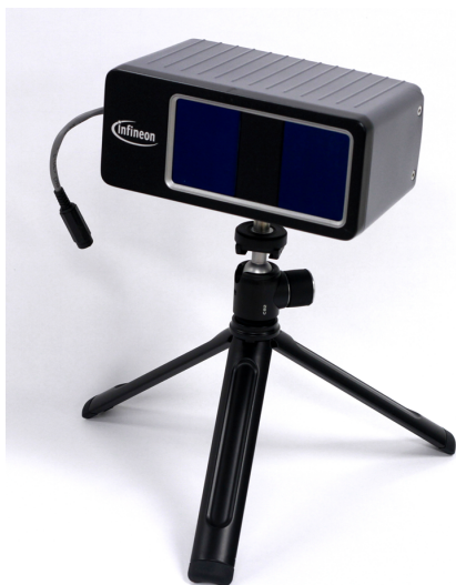
Figure 9. 1D MEMS mirror based LiDAR prototype.
