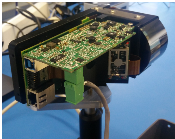
Figure 10. LiDAR prototype implementing optics, lasers, controllers, MEMS mirror, Receiver Circuits, MEMS Driver ASIC, and signal processing.
