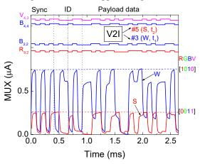
Figure 9. Proof of concept. MUX/DEMUX signals. V2I communication from Vehicles 1 and 2 and the infrastructure. On the top the transmitted channels packets [R, G, B, V] are decoded.
