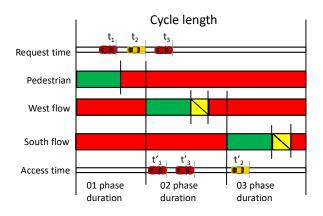
Figure 8. Phasing of traffic flows: phase number 01 (pedestrian phase), phase number 02 (W flow), phase number 03 (S flow).
