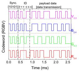
Figure 4. Frame structure. Representation of one original encoded message [10101: rrr ccc: XY....]. R<sub>3,4</sub>, G<sub>3,3</sub>, B<sub>2,4</sub> and V<sub>2,3</sub> are the transmitted node packet, in a time slot, from the crossroad in the network.
