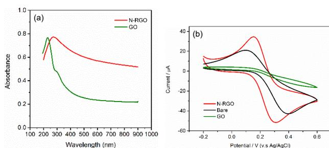
Figure 1. (a) UV-Vis spectra of GO and N-RGO, (b) Cyclic voltammograms of bare electrode, GO, and N-RGO in 0.1 M KCl solution containing 5 mM  $[\text{Fe}(\text{CN})_6]^{3-}/[\text{Fe}(\text{CN})_6]^{4-}$ .
