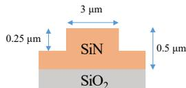
Figure 2. Waveguide structure
