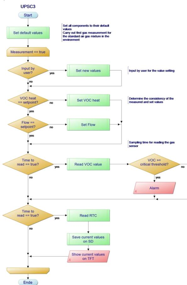
Figure 5. Main functions and the sequence of UPSC3
