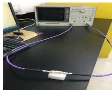
Figure 3. Measurement setup VNA HP 8753D connected to a microwave sensor via coaxial cable.
