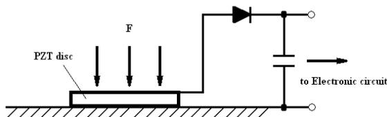
Figure 12. Mechanical force applied to a PZT disc followed by an energy converter.
