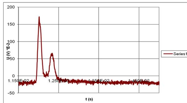
Figure 6. Electrical signal generated by a PZT core of 6 mm thickness hit by mechanical shocks.
