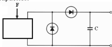
Figure 11. PZT element generator with diodes and parallel capacitor.
