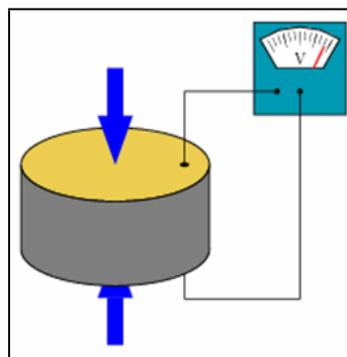
Figure 1. Piezoelectric generators principle.
