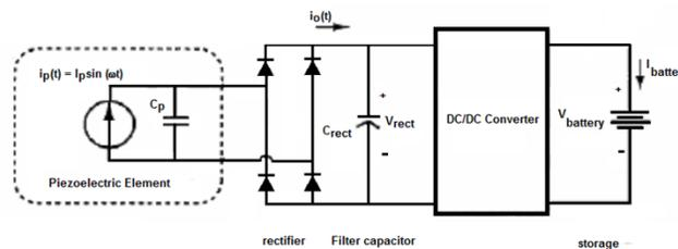
Figure 13. Typical energy harvesting circuitry.
