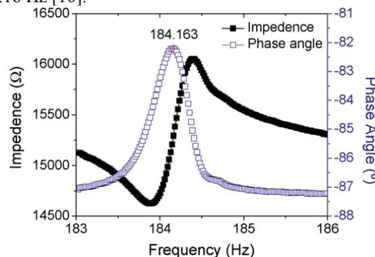
Figure 8. Measured resonant frequency of the PZT cantilever device [10].
