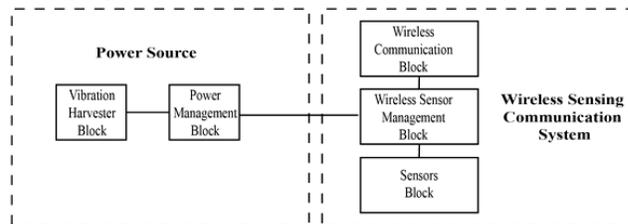
Figure 14. Block diagram of a wireless sensor node powered by a vibration energy harvester. [14]
