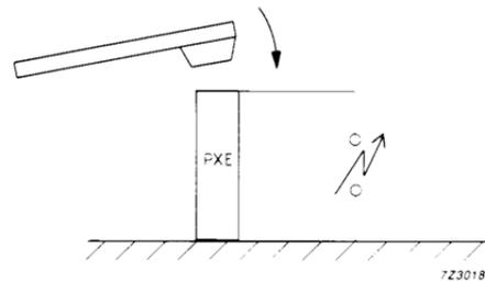
Figure 5. The principle of high voltage and spark generation [8].
