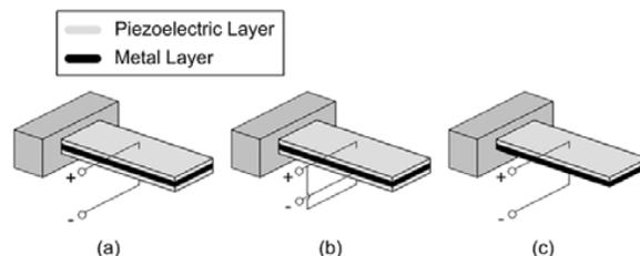
Figure 4. (a) A series triple layer type piezoelectric sensor. (b) A parallel triple layer type piezoelectric sensor. (c) A unimorph piezoelectric sensor [8].
