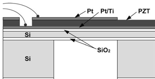
Figure 7. The schematic of the side view of a piezoelectric energy harvesting cantilever based on a silicon on insulator (SOI) wafer [9].
