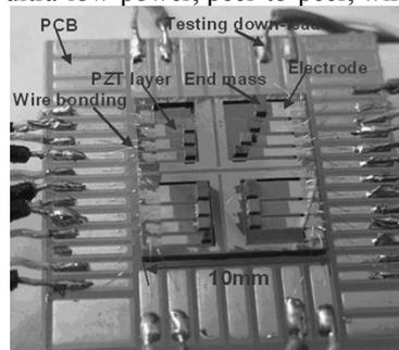
Figure 9. Picture of power generator array prototype [11].
