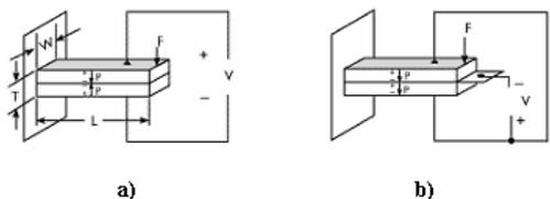
Figure 3. Series (a) and parallel (b) operation modes for bimorph actuators [2].
