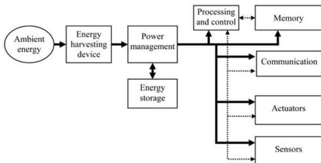
Figure 10. A generic sensor network node with energy harvesting device [13].
