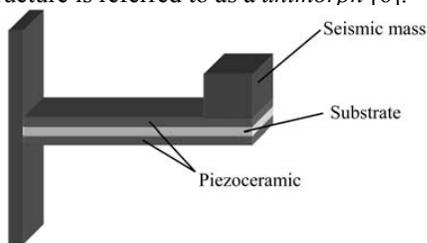
Figure 2. Piezoceramic cantilever resonator [6].
