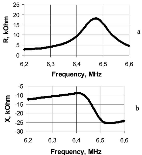
Figure 6. The frequency dependencies of the real (a) and imaginary (b) parts of the electrical impedance for the sensor loaded by gasoline with octane number of 95.
