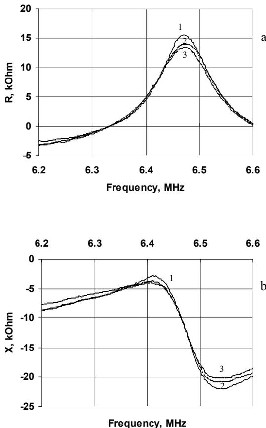
Figure 10. Theoretical frequency dependencies of real (a) and imaginary (b) parts of electrical impedance for permittivity 2.0 (1), 2.1 (2) and 2.2 (3).
