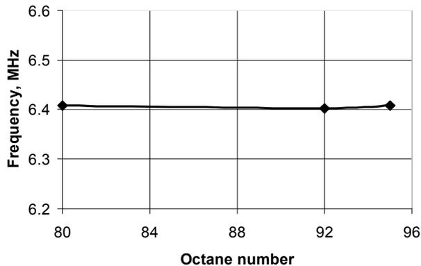
Figure 8. The dependence of the frequency of series resonance on octane number of gasoline.
