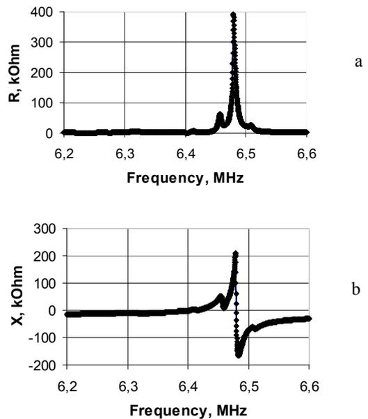
Figure 3. The frequency dependencies of the real (a) and imaginary (b) parts of the electrical impedance of the empty sensor
