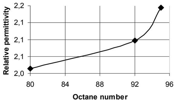
Figure 1. The dependence of measured permittivity of the gasoline on its octane number
