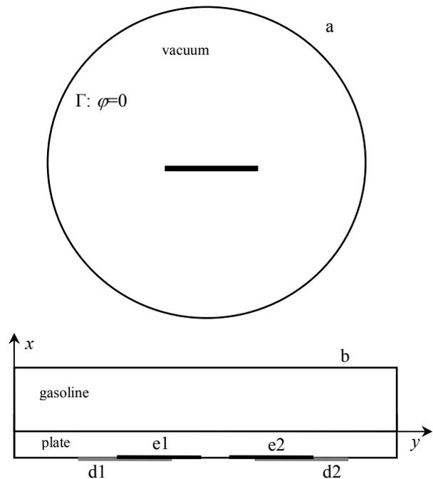
Figure 9. (a) Overview of the region of solution; (b) the central part of the region of solution: the plate of resonator and the gasoline layer, e1, e2 are electrodes, d1, d2 are damping layers.
