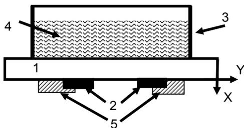
Figure 2. The gasoline sensor: 1 – piezoelectric plate, 2 – electrodes, 3 – liquid container, 4 – gasoline under study, 5 – damping layer.
