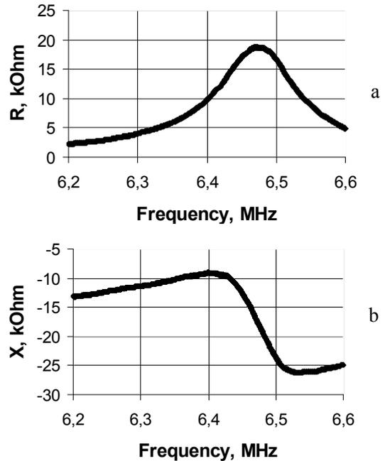
Figure 5. The frequency dependencies of the real (a) and imaginary (b) parts of the electrical impedance for the sensor loaded by gasoline with octane number of 92.
