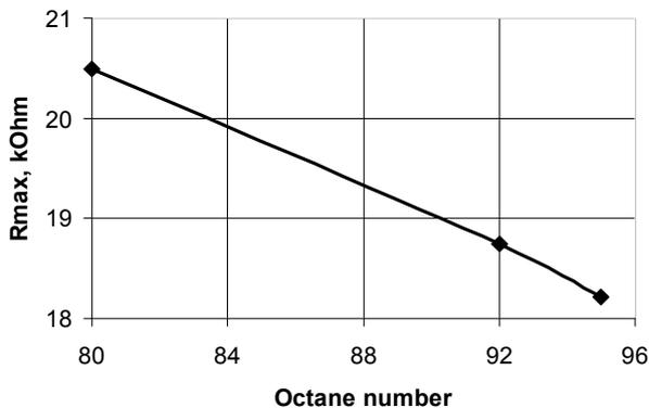
Figure 7. The dependence of the value of real part of the electrical impedance at the frequency of the parallel resonance on octane number of gasoline.
