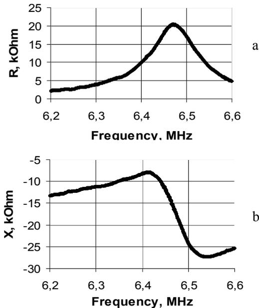
Figure 4. The frequency dependencies of the real (a) and imaginary (b) parts of the electrical impedance for the sensor loaded by gasoline with octane number of 80.
