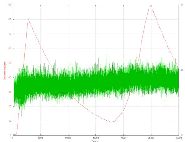
Figure 4. Phase response (green curve) with particle concentration variation (red curve) for a Rayleigh wave sensor.
