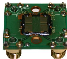
Figure 1. Surface Acoustic Wave sensor
