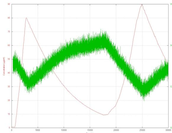
Figure 2. Phase response (green curve) with particle concentration variation (red curve) for a Love wave sensor with a photo-resistive resin guiding layer.
