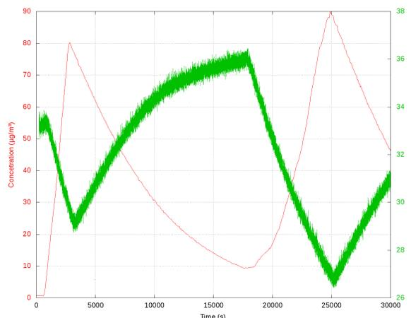
Figure 3. Phase response (green curve) with particle concentration variation (red curve) for a Love wave sensor with a 1.8  $\mu\text{m}$  silica guiding layer.
