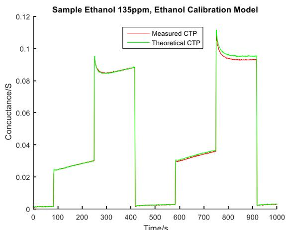
Figure 2. Comparison of measured CTP and theoretical CTP based on the ethanol calibration model for sample ethanol 135ppm.
