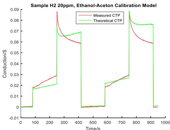
Figure 6. Comparison of measured CTP and theoretical CTP based on the ethanol-acetone calibration model for sample H2 20ppm.
