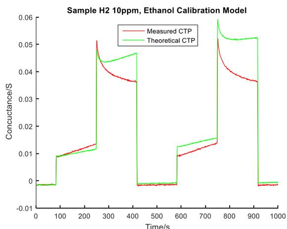
Figure 4. Comparison of measured CTP and theoretical CTP based on the ethanol calibration model for sample H2 10ppm.
