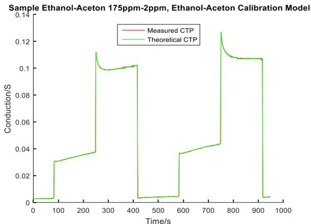
Figure 5. Comparison of measured CTP and theoretical CTP based on the ethanol-acetone calibration model for sample ethanol 175ppm acetone 2ppm.
