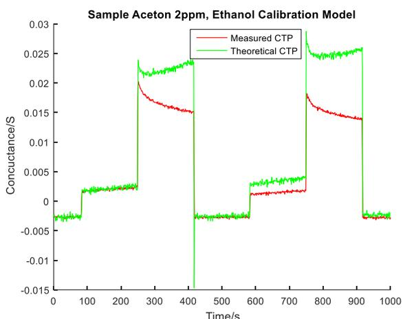
Figure 3. Comparison of measured CTP and theoretical CTP based on the ethanol calibration model for sample acetone 2ppm.
