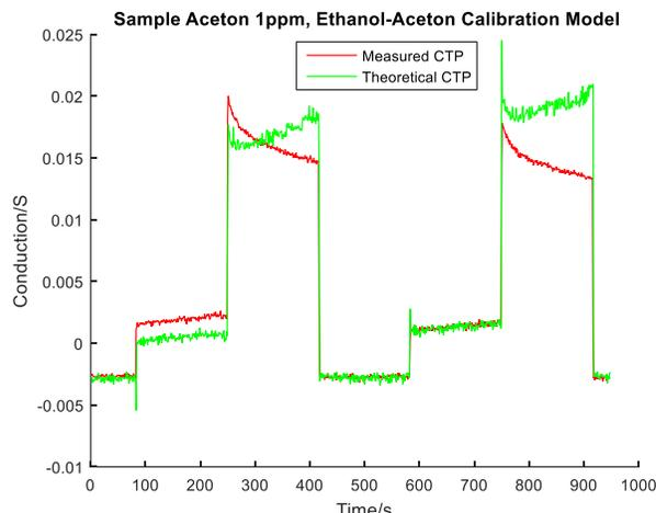
Figure 7. Comparison of measured CTP and theoretical CTP based on the ethanol-acetone calibration model for sample acetone 1ppm.
