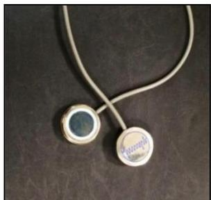
Figure 1: PS25015A Dry Electrodes
