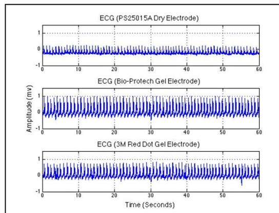
Figure 4: ECG signals acquired from the three electrodes
