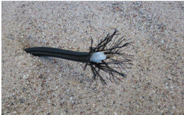
Figure 6: Prototype of the sensor enabled RFID tag.
