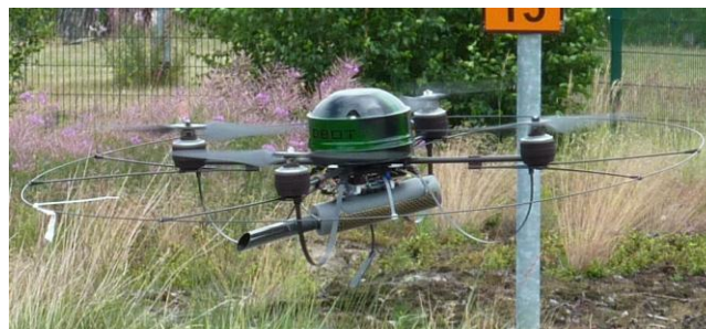
Figure 3: Micro-drone with multi-sensor equipment in flight.
