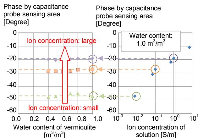
(a) Vermiculites were interfused with three solutions with different ion concentrations. Experiment of the relationship between water content and phase.
