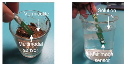
(a) The picture shows a photo of a water content experiment using vermiculite, as shown in Fig. 4 (a) and Fig. 5 (a).
