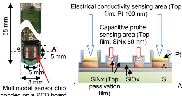
(a) The picture shows a multimodal sensor. The sensor has a small chip size, and is bonded on a PCB board that is inserted into the beds.
