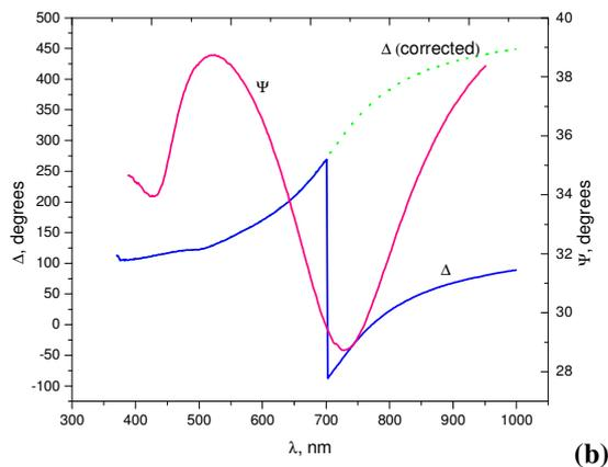
Fig. 1. (a) TIRE experimental set-up. (b) Typical TIRE spectra of  $\Psi$  and  $\Delta$  measured on bare surface of gold. Dotted line shows corrected (by adding  $360^\circ$  to negative values) of  $\Delta(\lambda)$  spectrum.
