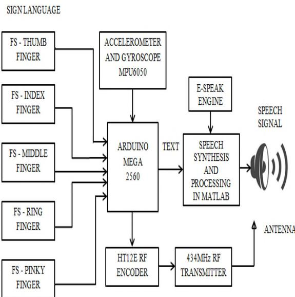
Figure 2. Block diagram of Sign to Speech system.
