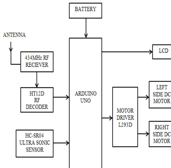
Figure 3. Block diagram of Sensor Controlled Wheelchair.
