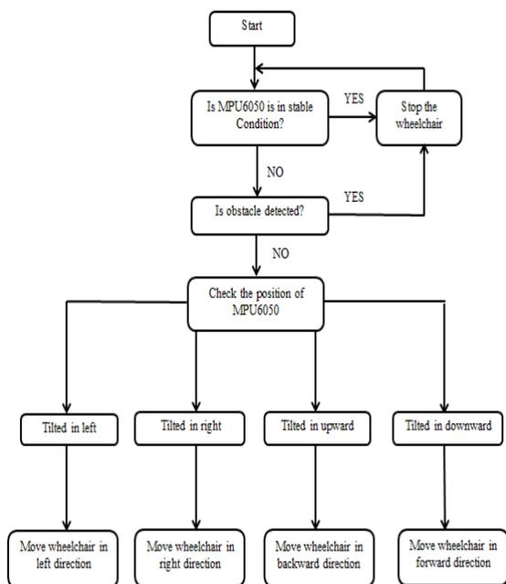
Figure 5. A flowchart of Sensor Controlled Wheelchair.
