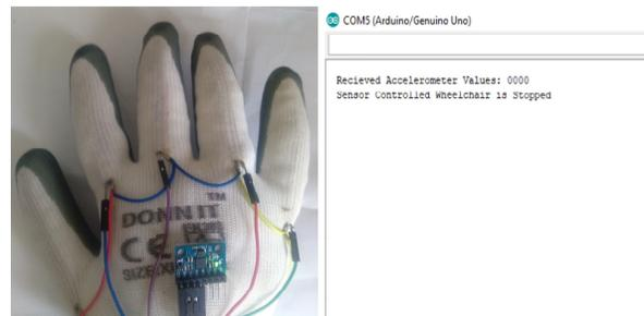
Figure 16. Sensor Controlled Wheelchair is Stopped
