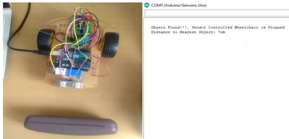
Figure 11. Object Detection in Sensor Controlled Wheelchair
