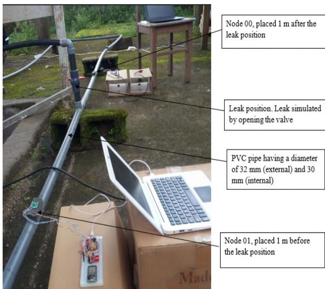
Figure 1. A cross-sectional view of the laboratory testbed.
