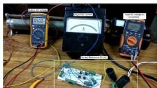
Figure 12. Measurement set-up for constant DC current source
