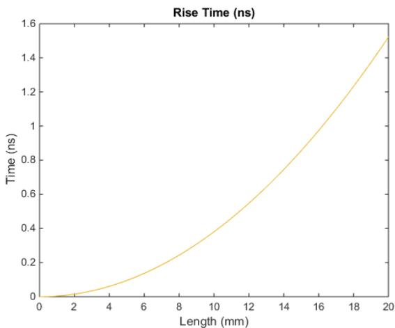
Figure 6. Rise Time of a signal seen across a pixel row through a metal line of up to 20 mm and a pixel pitch of 35  $\mu\text{m}$  with the following parameters:  $\rho = 2.65 \cdot 10^{-8} \Omega \cdot \text{m}$ ,  $T = 425 \text{ nm}$ ,  $C_{\text{pixel}} = 2 \text{ fF}$ ,  $C_{\text{surface}} = 0.015 \text{ fF}/\mu\text{m}^2$ ,  $C_{\text{edge}} = 0.032 \text{ fF}/\mu\text{m}$  and  $w = 3 \mu\text{m}$ .
