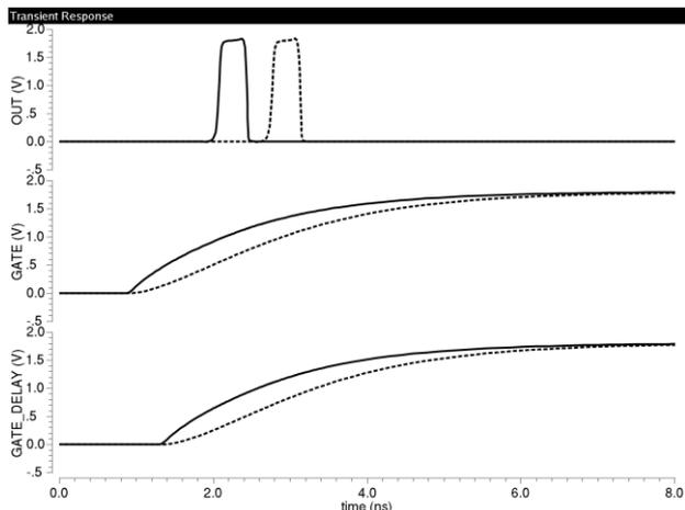
Figure 11. Simulation of a 300 ps pulse created using the edge-based technique (line: 20 mm length,  $3 \mu\text{m}$  width). Signals at the beginning of the line (solid line) and at the end (dotted line)
