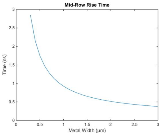
Figure 7. Rise Time with respect to metal track width at midway along a row of pixels
