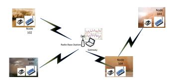
Figure 3. Wireless Dust Measurement System Architecture
