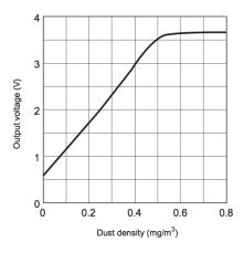
Figure 8. Dust Sensor Output Characteristic
