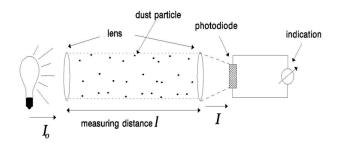
Figure 1. Optical Dust Measurement Principle Schematic
